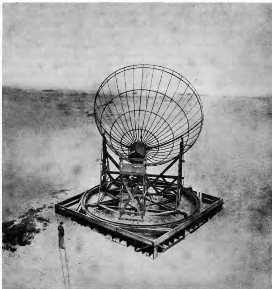
One of the large parabolic reflectors used by Frederick A. Kolster in 1928 for a series of experiments with directional antenna systems employing short waves. These experiments led directly to later developments in microwave directional transmission.
